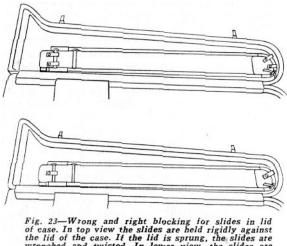
Fig. 23—Wrong and right blocking for slides in lid of case. In top view the slides are held rigidly against the lid of the case. If the lid is sprung, the slides are wrenched and twisted. In lower view, the slides are held loosely against the lid so that though the lid is sprung or twisted, the single button across the brace and crook gives the slides enough freedom so they are not twisted with the lid.
