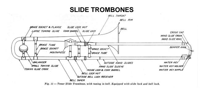
**Why Hand Slides Require Careful Handling.** The hand slides of the slide trombone are delicate and require care- ful handling. The brass outside slides have a wall thickness of from .011" (11 thousandths of an inch) to as little as .006" (6 thousandths of an inch), on the lightweight models.
