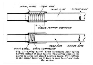
Keep the tuning slide clean and lubricated. Use vaseline or tallow on the slides and they will work more freely and cause less trouble. After applying the vaseline or tallow, push the slides all the way in and wipe off the excess which squeezes out at the joint.
