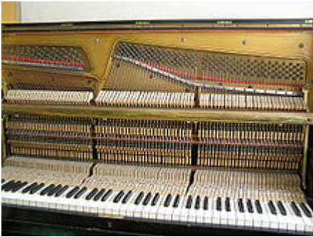
The mechanism and strings in upright pianos are perpendicular to the keys.
