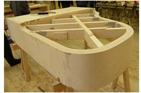
Outer rim of Estonia grand piano during the manufacturing process
