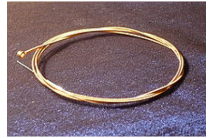
A wound acoustic guitar string (phosphor bronze wound around steel) with a ball end, 0.044" gauge
