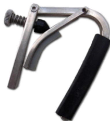
A Shubb capo, which uses a lever-operated over-centre locking action clamp
