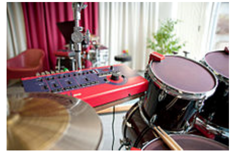
Triggers sensors in use, here they are red and mounted on the rims of the snare drum, bass drum and hanging toms. The larger box in the same colour red is the "brain" to which they are connected.
