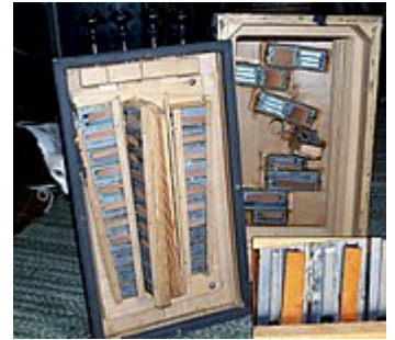
Accordion reed ranks with closeup of reeds
